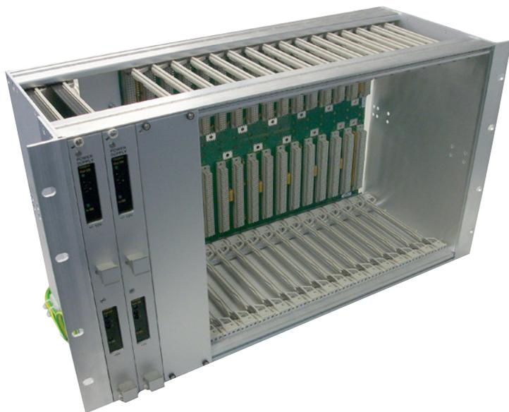
**Integrated 6U x 84HP x 180mm KM6-HD IEC sub-rack , wired with VMEbus backplane & custom H15 power supplies - simulation application.**
